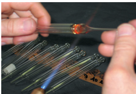
Photos 6 and 7: preparing the blank for dipping
